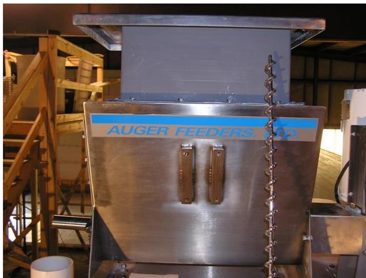
**Figure 6: Photograph Showing Variable-speed Auger Feeder**
