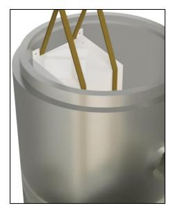
Gently slide the HydroDome outlet stub into the manhole outlet as far as possible without forcing it, until the HydroDome insert is close to the wall.
