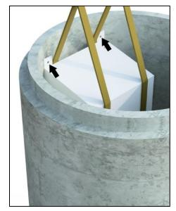
Drill 0.5" holes, no more than 3" into the manhole wall, through the holes in the attachment tabs.
