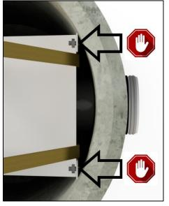
Use the supplied stainless steel concrete anchor bolts, washers and nuts to fasten the HydroDome flanges to the structure wall. STOP TIGHTENING AS SOON AS BOLT MEETS PLASTIC. DO NOT OVERTIGHTEN.
