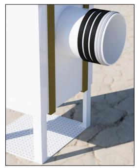
Apply two generous beads of Pro-Seal34 caulk around the outlet stub of the HydroDome insert directly next to the weather stripping furthest from the back of the HydroDome.
